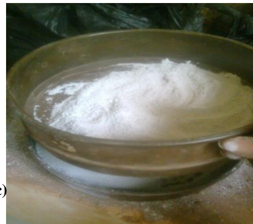
Plate 1: (a) Raw cow bone dumped as waste at Ikpa market Nsukka. (b) washed and sun-dried cow bone (c) ground and sieved cow bone particles
