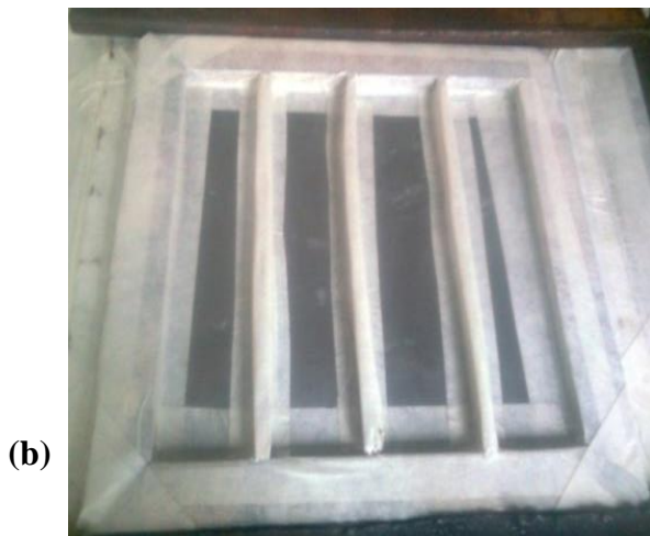
Plate2: Moulds for producing (a) Tensile Specimens (b) Compressive and impact specimens
