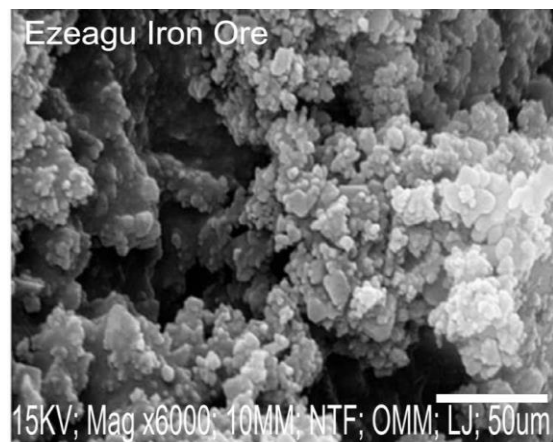
Figure 3b: SEM image at 50 microns and x 6000
