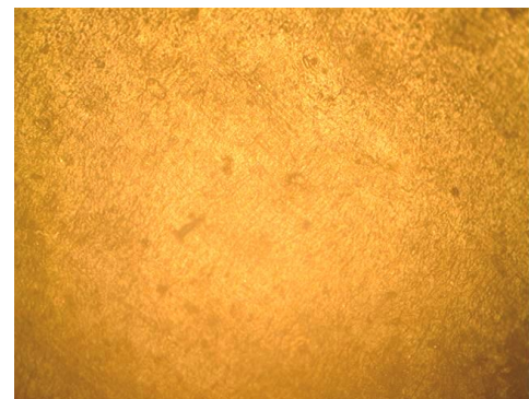
Plate. A3: Microstructure of 20wt% BDS (90 \mu m) reinforced HDPE (x100).
