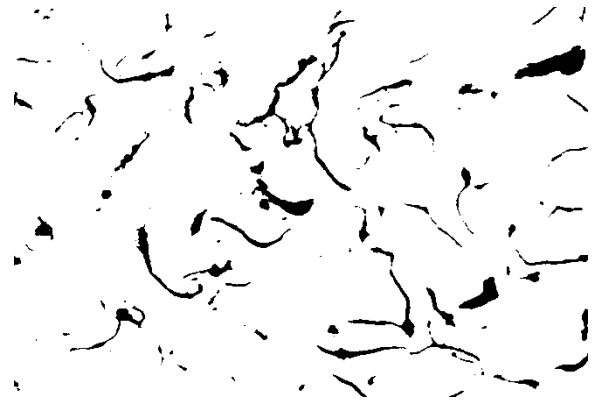
Plate 3: Microstructure of Sand Cast Grey Iron of Diameter 25 mm showing Graphite Flakes breaking the continuity of the Ferrite Matrix Type A flakes (x100). Etching time 10 seconds.
