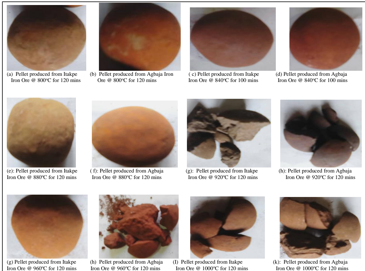
Figure 12 (a – k): Images showing the reducibility of both pellets at temperature from 800°C -1000°C for 120mins
