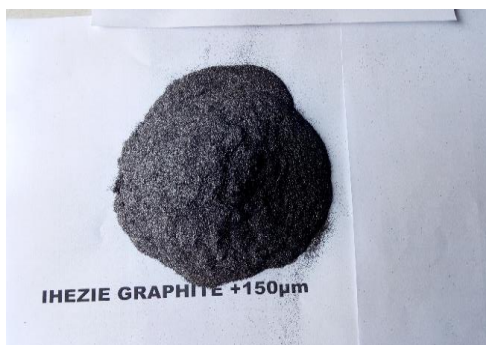
Figure 9 Photograph of processed Taraba Upland graphite of particle size 150 \mu m (98.87%FC).
