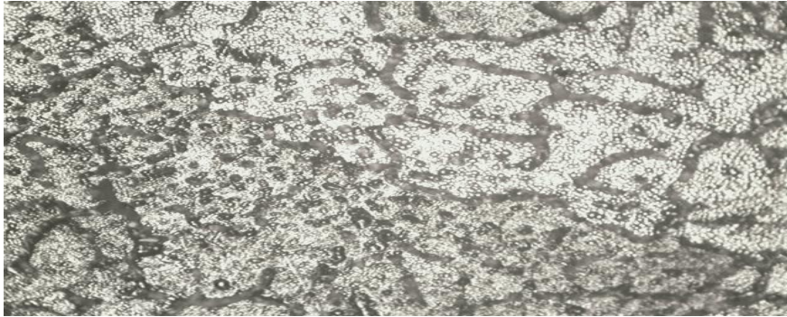
Plate I: Micrograph of unreinforced as-cast Al-Si-Mg alloy, showing magnesium silicide, ( Mg_2Si ) (black) and \alpha -Al matrix (white). \times 100 , acid etchants (0.5ml HF acid and 99.5ml distilled water).
