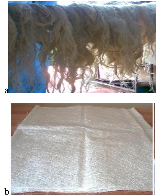
Plate 1: (a) processed sisal fiber and (b) random E-glass fiber mat
