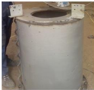
Fig. 4: Fabricated atomizing chamber
