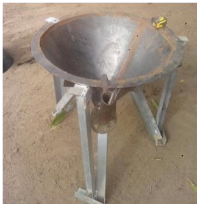
Fig. 5: Fabricated collector chamber
