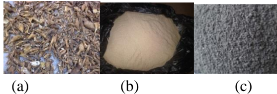
Fig.1. Photographs of the cassava cortex: (a) cassava cortex under sun drying (b) sieved uncarbonized cassava cortex (c) sieved carbonized cassava cortex.
