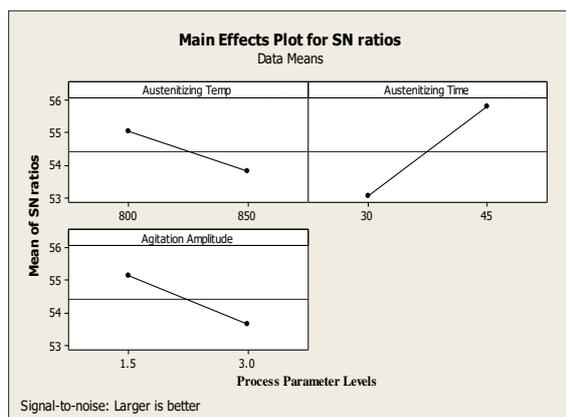
**Figure 8:** Impact of process parameters on mean S/N ratio of Hardness of High carbon steel quenched in FM
