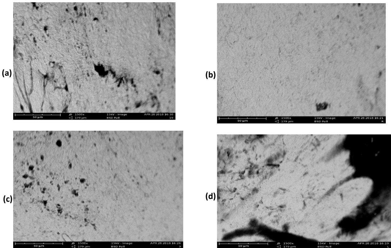
Plate 2: SEM Image of sample quenched in a) EM, b) ETM, c) TM and d) FM at optimum parameters setting
