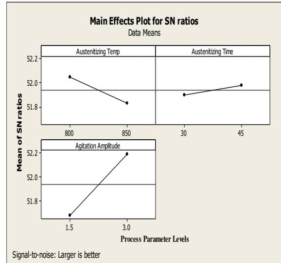
**Figure 9:** Impact of process parameters on mean S/N ratio of Hardness of High carbon steel quenched in SAE40
