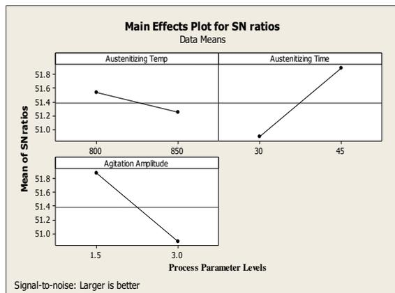
**Figure 7:** Impact of process parameters on mean S/N ratio of Hardness of High carbon steel quenched in EC
