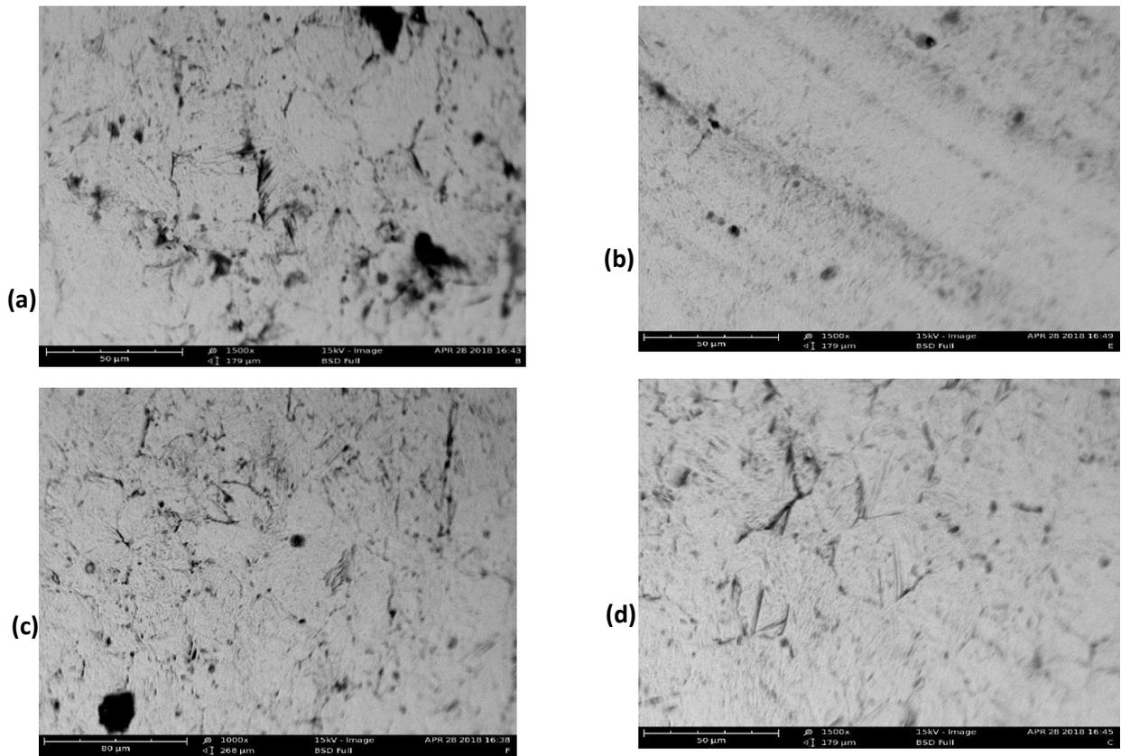
Plate 1: SEM Image of sample quenched in a) EC, b) ETC, c) TC and d) FC at optimum parameters setting
