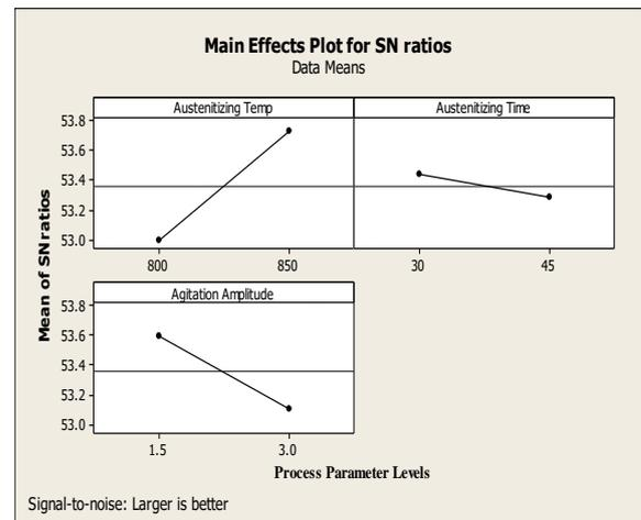
**Figure 2:** Impact of process parameters on mean S/N ratio of Hardness of High carbon steel quenched in TC
