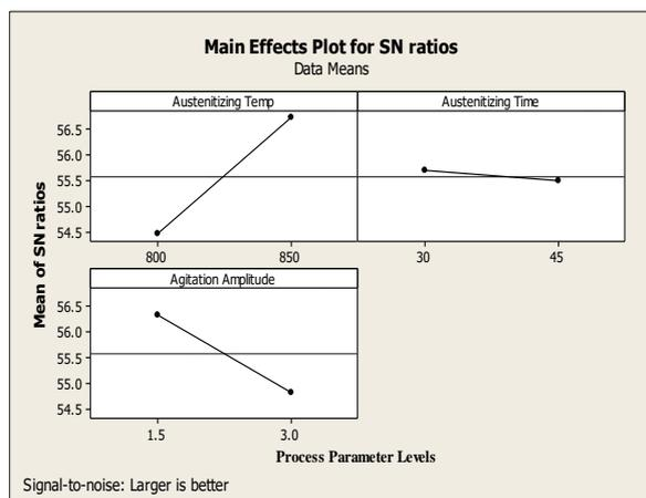
**Figure 1:** Impact of process parameters on mean S/N ratio of Hardness of High carbon steel quenched in ETC
