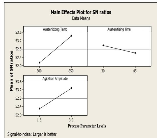
**Figure 3:** Impact of process parameters on mean S/N ratio of Hardness of High carbon steel quenched in TM
